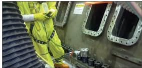
**SAFE BOLTING:** Exposure to high pressure bolting equipment is a thing of the past. Hands-Free Remote Operation on horizontal, vertical and inverted applications.
