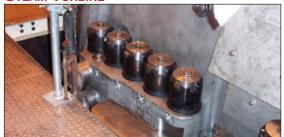
IN SERVICE FOR 14 YEARS WITH THE HYTORC-NUT DISASSEMBLY TIME, FREE OF INJURY: 4 HRS 26 MIN. ASSEMBLY TIME WITHOUT A SINGLE NUT REPLACEMENT: 3 HRS.
