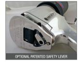
This safety mechanism drastically reduces operator error. The lever must be depressed while pulling the trigger, ensuring operator keeps hands away from pinch points.
